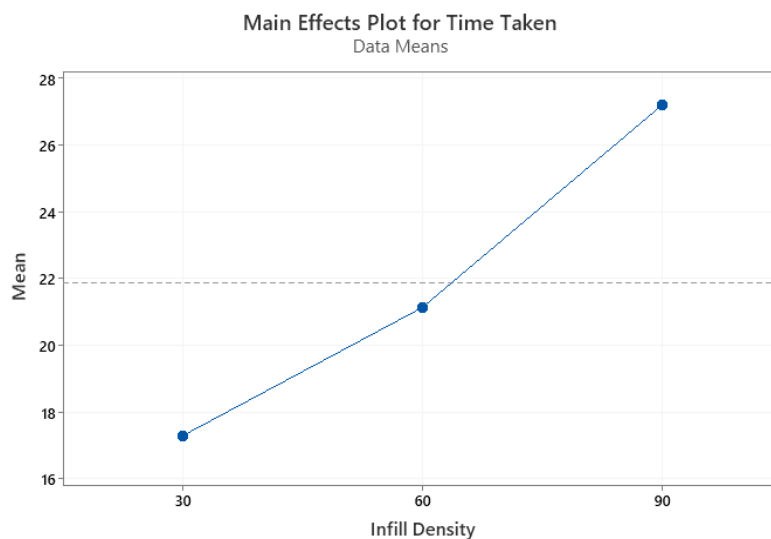
Fig. 8. Relationship Between Infill Density and Shape Recovery Time
